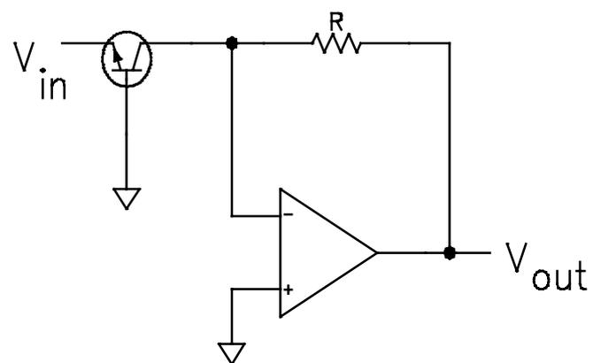
$$V_{out} = I_o R e^{-q \frac{V_{in}}{kT}}$$
