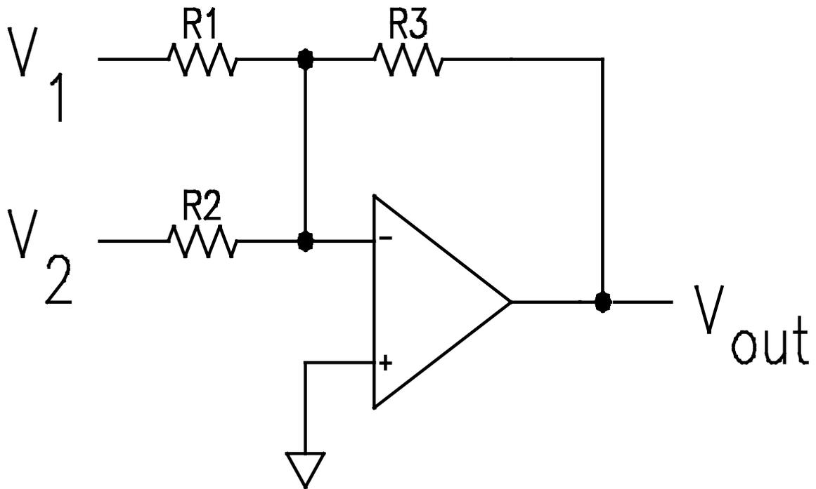
$$V_{out} = - \left( \frac{R_3}{R_1} V_1 + \frac{R_3}{R_2} V_2 \right)$$
