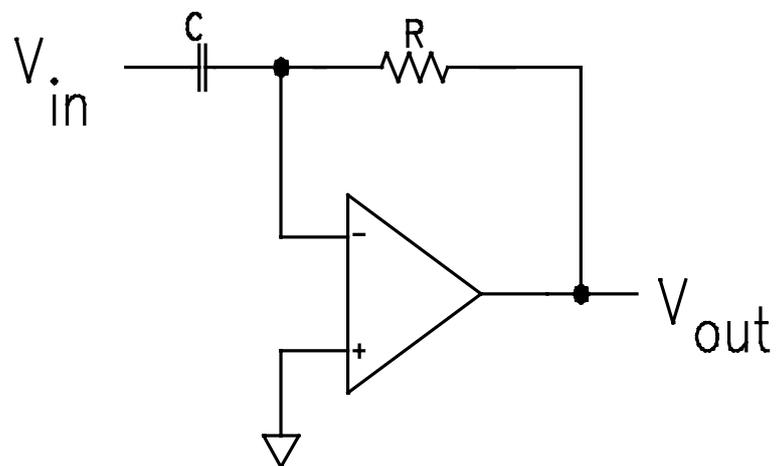
$$V_{out} = -RC \frac{dV_{in}(t)}{dt}$$
