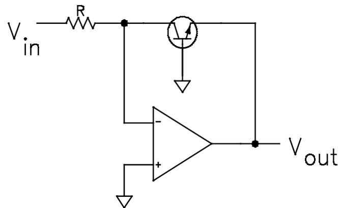
$$V_{out} = -\frac{kT}{q} \ln \frac{V_{in}}{I_o R}$$
