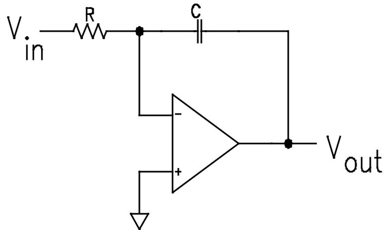
$$V_{out} = -\frac{1}{RC} \int V_{in}(t) dt$$
