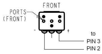
4-20mA sensor connector pinout
